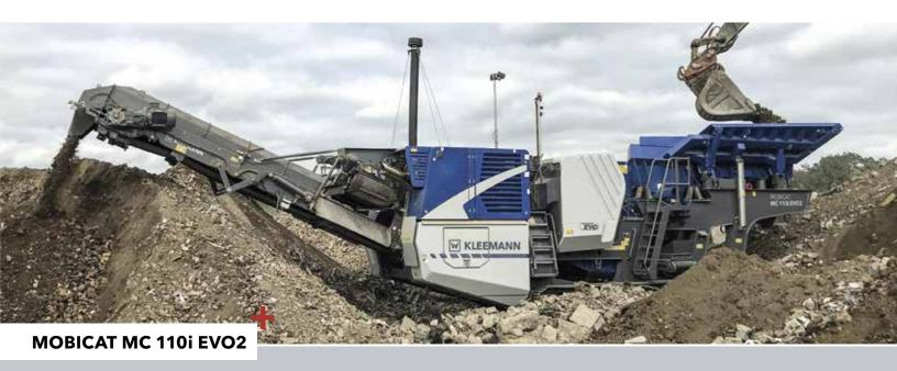
The jaw crusher MOBICAT MC 110i EVO2 is used for the pre-crushing of almost all natural stones and in recycling. Compact dimensions, efficient prescreening, simple operation via SPECTIVE and impressive production outputs characterize this efficient key player.
