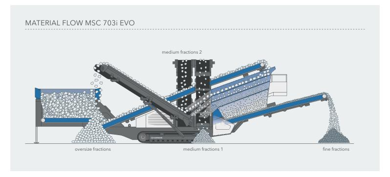
The material flow of the MSC 702i and MSC 703i EVO is designed for a high output. Starting with the feed hopper, which has an impressive holding capacity and which widens in material direction of flow. The material is thus transferred via the hopper discharge conveyor with optimized distribution onto the extra-wide feeding conveyor. Thanks to impact plates on the belt discharge and screen casing loading, the material is distributed evenly on the generously
