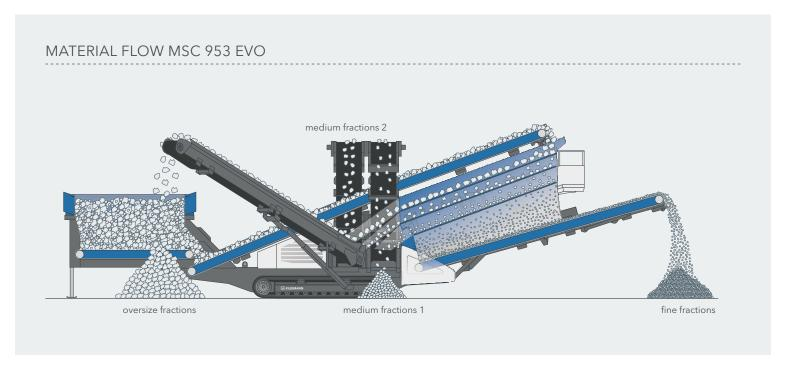
Thanks to compact transport dimensions, short set-up times and a large selection of screen surfaces, the classifying screening plants MSC EVO can be used flexibly. For efficient processing of large volumes, the design of the material flow has been optimized: starting with the feed hopper that widens in the material direction of flow, to the wide feeding
