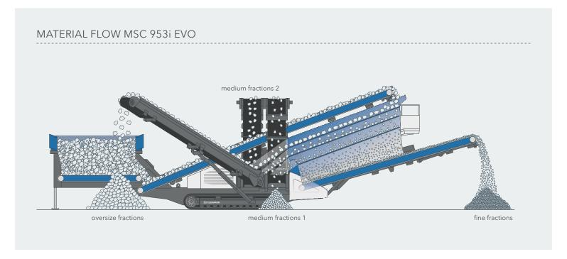
Thanks to compact transport dimensions, short set-up times and a large selection of screen surfaces, the classifying screening plants MSC EVO can be used flexibly. For efficient processing of large volumes, the design of the material flow has been optimized: starting with the feed hopper that widens in the material direction of flow, to the wide feeding
