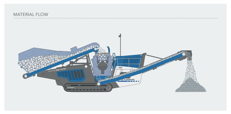
The MOBICONE MCO 110i PRO is equipped with a simple sliding mechanism on the feed unit, which puts the machine into a compact transport position and enables quick set-up. The sliding mechanism also makes it easy to adjust the material discharge pattern into the crusher - for optimal loading. Fitted with the "Tramp Release" and
