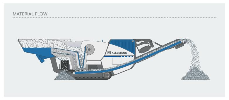
With its low weight and very compact dimensions, the MOBICAT MC 100i EVO can be used directly on site – even at narrow or hard-to-reach construction sites in urban areas. Short set-up times are also ensured thanks to feeding unit integrated in the chassis, which means that it no
