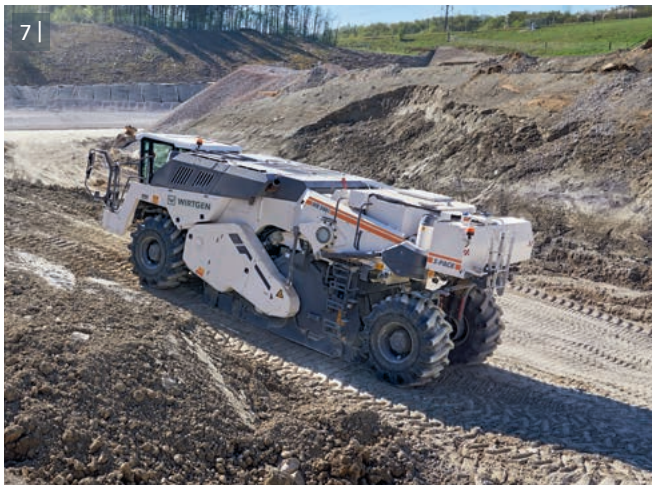
7 | The "S-Pack" (short for "spreader pack") binding agent spreader optionally built into the soil stabilizer is used for dust-free binding agent discharge.
