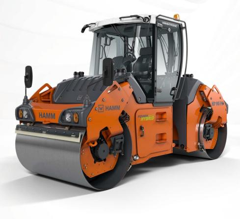
Tandem rollers Series HD+ Tandem roller with two vibrating roller d H276
