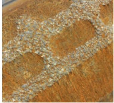
> *Different arrangement of the ceramic inserts in the basic material*
