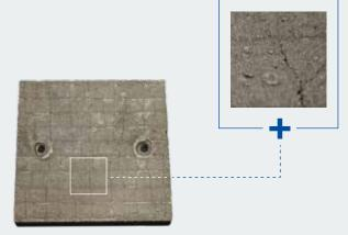
Surface of plates for inside of crusher. Cracks are a prerequisite for optimal hardness.
