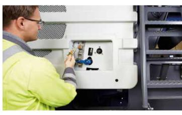
> If keys are removed, the rotor remains safely locked.
