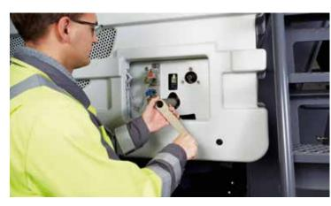
> The rotor locking and turning device is enabled and can be moved with a crank.
