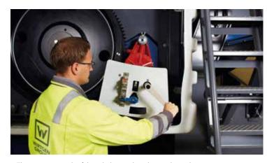
> The rotor is turned safely with the crank and moved into the optimum position for rotor ledge replacement.
