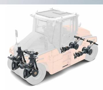
Of course, the braking power of the HP series pneumatic tyre rollers can be applied with great sensitivity because the electronically assisted drive control ensures gentle braking and acceleration the basis for smooth asphalt paving with no bumps or hollows.
