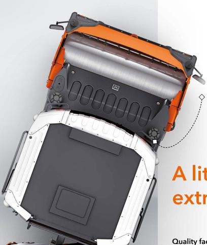
The turning circle of the HD+ is remarkably small. This means that even the large models can manoeuvre well in tight spaces, too.
