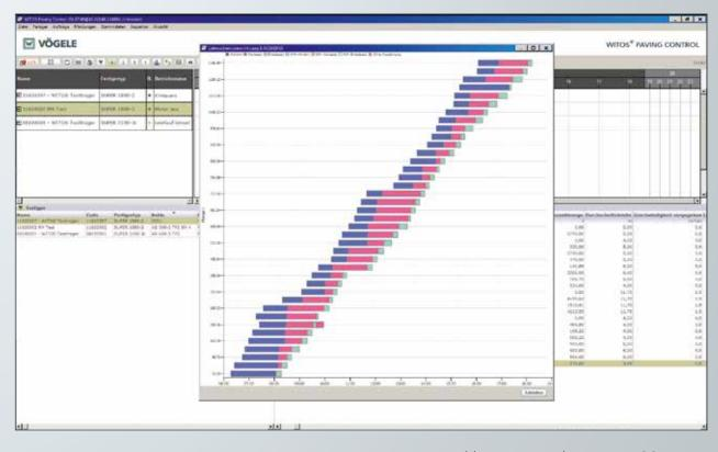
In addition to easy planning, WITOS Paving Control also monitors operations at a current job site. For example, the supply chain can be checked at any time.
