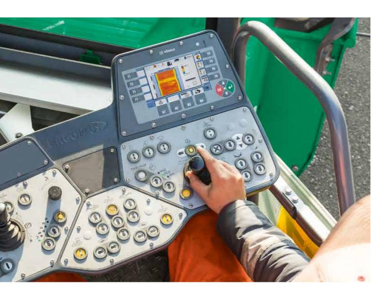
**The paver operator** is linked to the job site module via the ErgoPlus 3 display. For example, he can access current information on the job site and the progress of the project at any time. Thanks to clearly arranged and easily comprehensible diagrams, he can immediately recognize a deviation of the actual situation from the plan.
