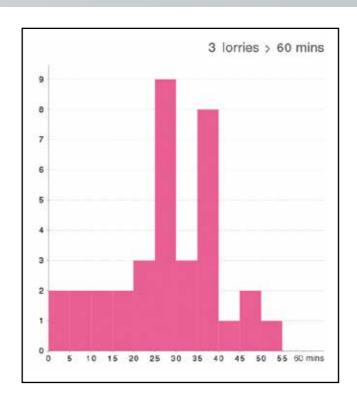
Comparing the arrival, waiting and unloading times of the lorries with the data on paving temperatures reveals weak points in the delivery chain.
