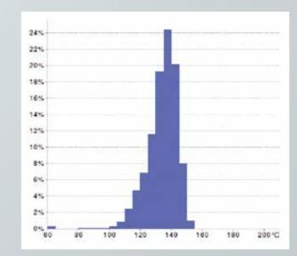
The bar chart on the left shows that 98% of the paved material was within the target temperature range.
