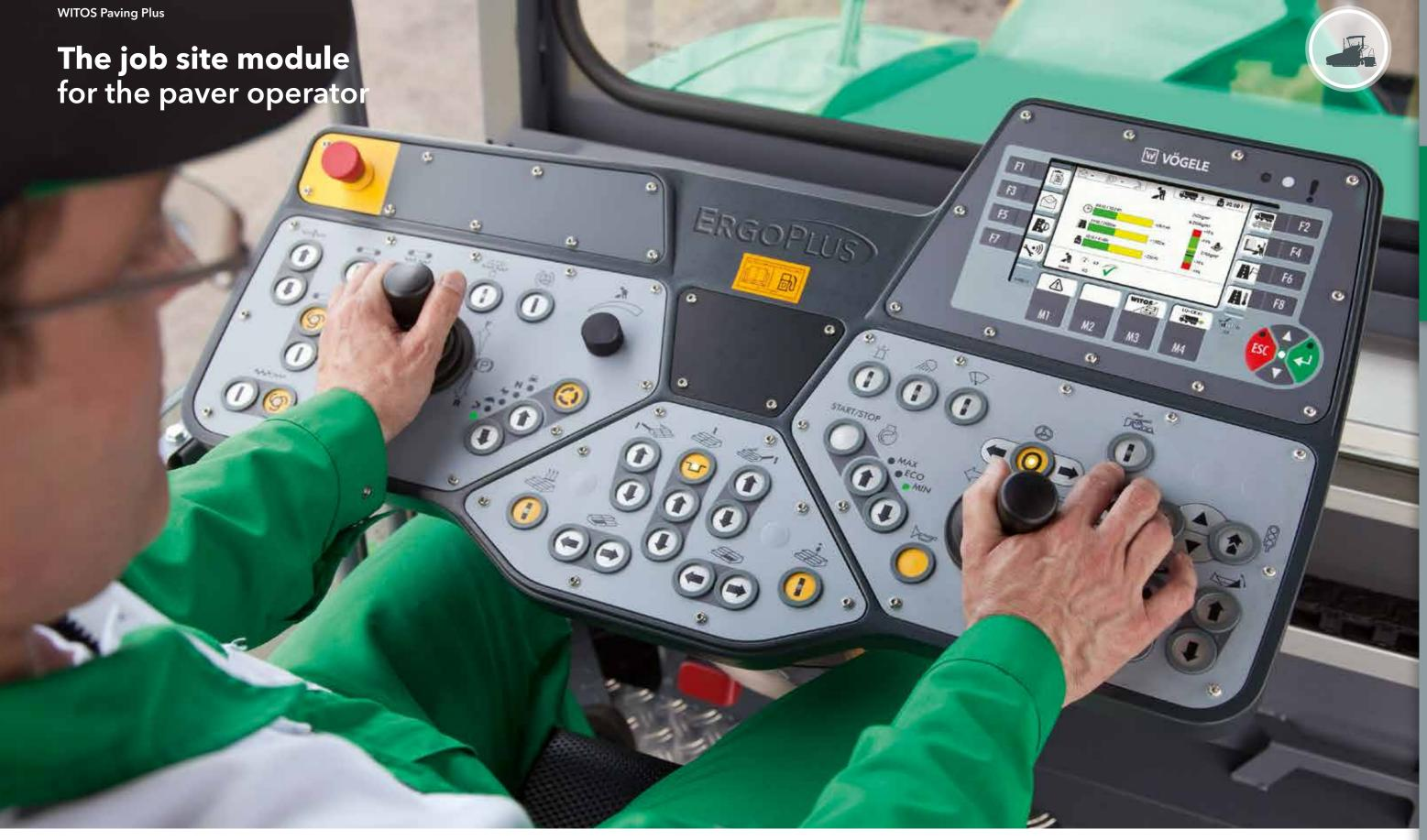
**The job site module** is an integral part of the VÖGELE ErgoPlus 3 paver operating system and offers the paver operator a unique tool for control and process optimization.
