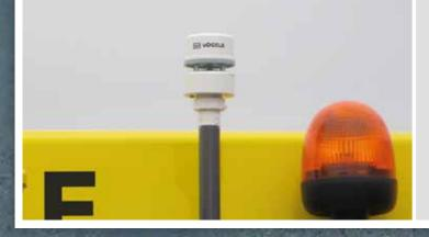
Along with the asphalt temperature, a weather station can also document the wind speed, wind direction, ambient temperature, air pressure and humidity.
