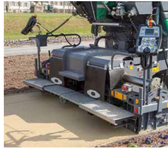
AB 340 V built up with 25cm bolt-on extensions
