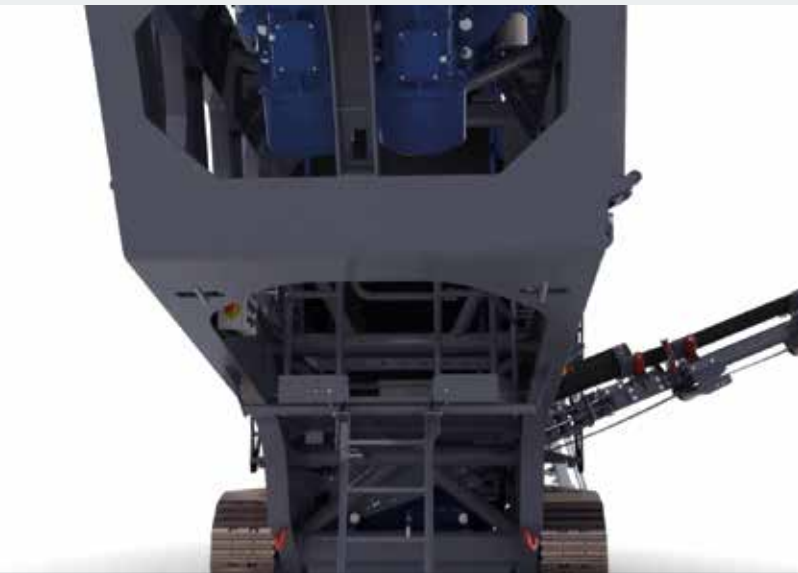
> MC 120i PRO – convenient screen surface changes thanks to ease of access
