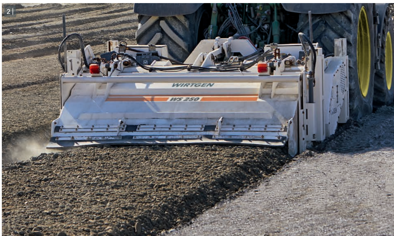
2 | Flawless mixing results and perfect leveling are the hallmarks of the tractor-towed stabilizer.
